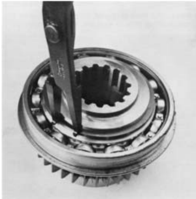
4. Remove snap ring from auxiliary drive gear.
