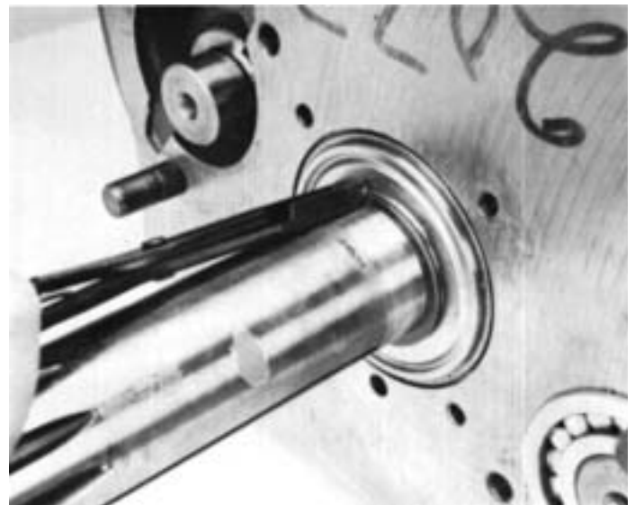
11. Install the bearing retainer snap ring.
