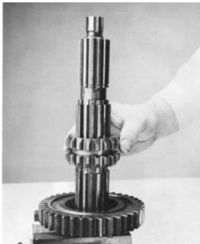
11. Remove Lo and reverse speed sliding clutch.
