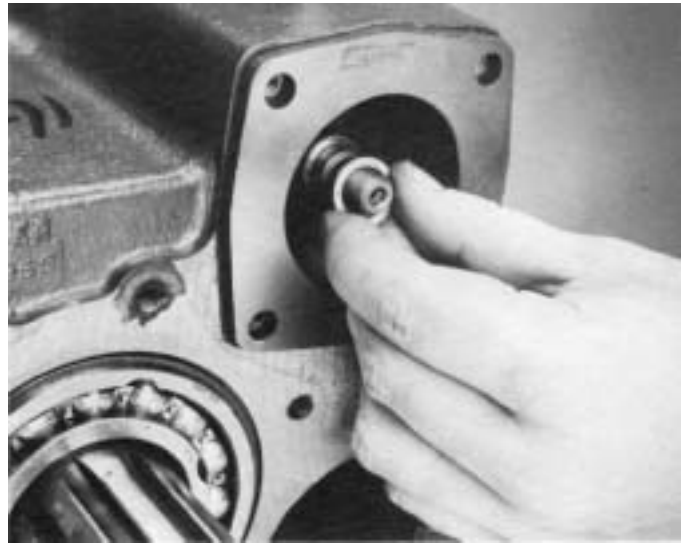
5. Remove the copper gasket from yoke bar.
