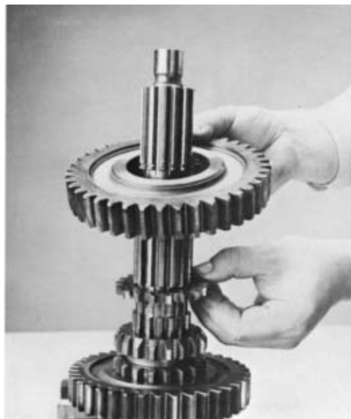
10. Remove Lo speed gear and tolerance washer.
