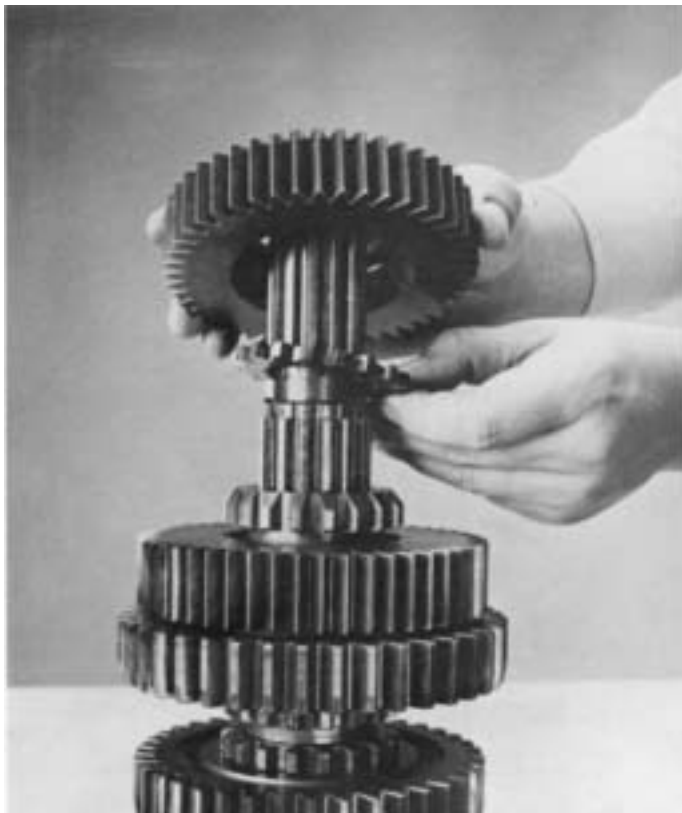
6. Remove the 2nd speed gear and tolerance washer.
